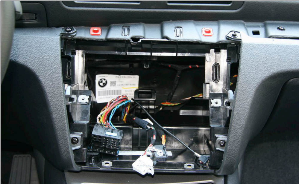
9. Remove out OEM head unit
